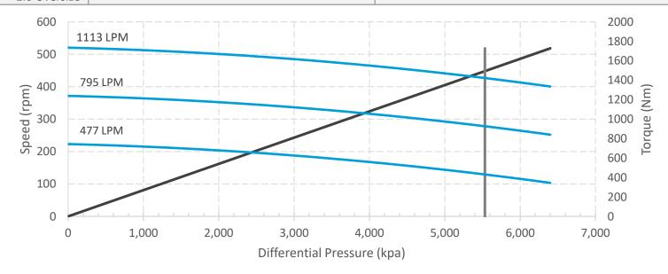
Power section performance curves are for reference only. Actual performance will vary with different downhole conditions and rotor/stator fits. If operated above the optimal differential pressure, stator life will be reduced. Optimal load power calculation is based on maximum RPM and optimal load torque. Information contained in this document is subject to change without notice.
